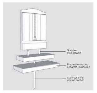
**Ground Anchor Fixing Method**
